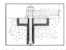
NORDBAK<sup>®</sup> Deep Pour Grout demonstrated its effectiveness in grouting a 12-cylinder, 3700-hp diesel engine and a 2650-kW generator successfully. The engine, weighing 52 tons, and the generator, along with its outboard, weighing 20 tons, were carefully positioned. Levelling shims were initially placed along the bottom of the foundation
